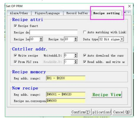
Automatic matching using link2 scanner: The data setting of the current recipe is read by the link2 scanner.
