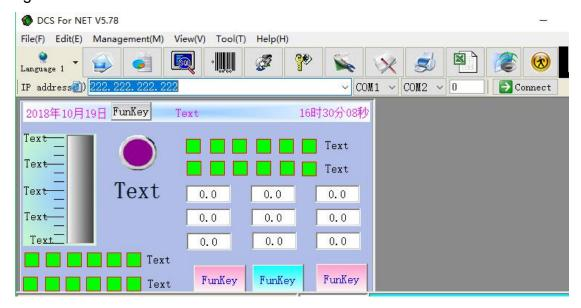
Among them, when using the touch screen download line for Ethernet monitoring, the IP address is set to "222.222.222."
