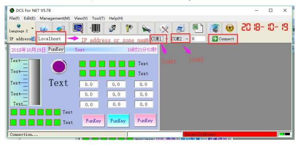
Note: During online simulation, the user password does not match the password set on the touch screen. Administrators must log in before modifying the encrypted register parameters.
