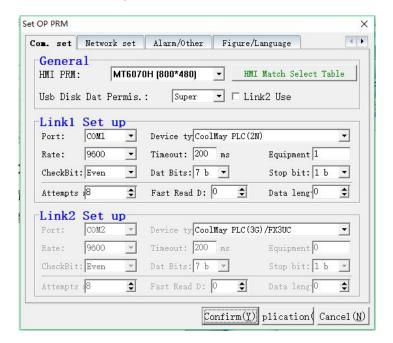
•HMI parameter: select resolution according to different HMI.
