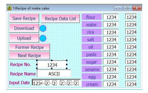
Through the relevant function settings in the function keys, buttons can be created on the screen to write each group recipe to the PLC and read the recipe from the PLC, save the recipe, and select the previous recipe and the latter recipe.
