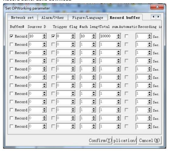
In the settings of historical data display module, record buffer zone must be assigned so that on-line interaction can be applied. Record buffer zone is the BACKUP RAM location where sampling data is stored. The location and size of record buffer zone must be set in advance.
