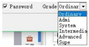
The supervisor password defaulted by the system is the same with the default password when updating program. The default password of others like common, manage, system, middle,advance is "12345678", when the default password is successfully log in, new password can be set.
