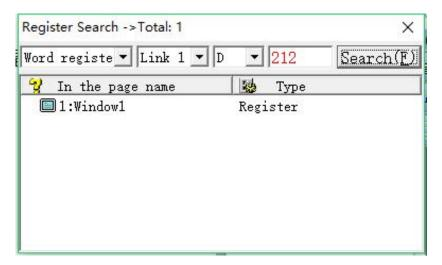
When using this function, first set the basic conditions of the registers you want to find, and then click the [Find] button. The searched component will be displayed in the output bar. Double-click an option in the output bar and the cursor will be automatically selected to the component.
