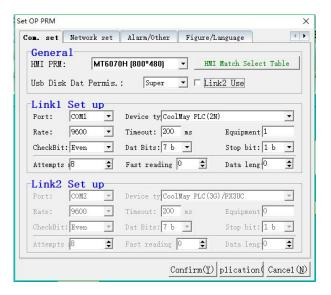
Set HMI parameters, Link1/Link2 COM port and PLC model, then click [Confirm].
