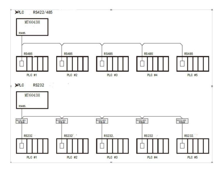
➤RS485/CAN\_Bus multi-controller communication. Initial ID address of extension
