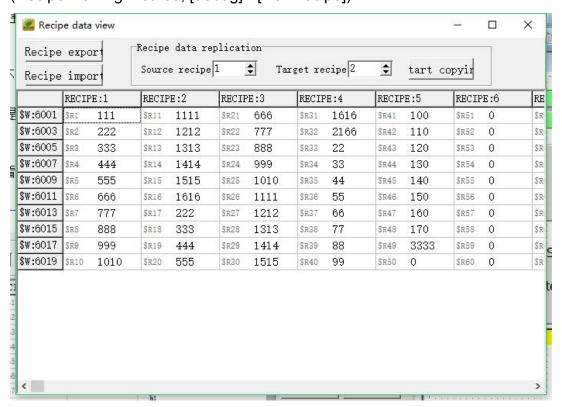
This recipe has 4 subsidiary recipes, each recipe has 10 members, its saved address is HMI's memory address from LW6001 to LW6010.
