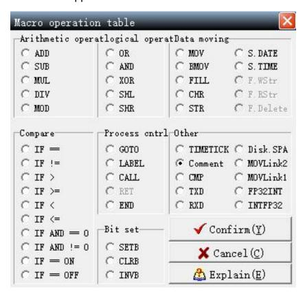
At this time, The user just move the mouse to the position of the desired command and press the OK button to return. Then click the [A1] [A2] [A3] button to edit the macro, that is, set the selected macro parameters.
