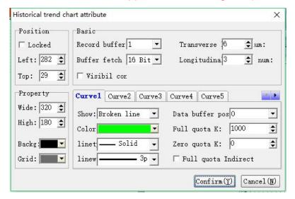
Historical trend graph: HMI can set sampling time and conditions to read numeric data of buffers which is designated by PLC, and store these data in the record buffer of HMI. After everlastingly and chronically sampling, the data will be convert to curve and displayed on the screen of HMI.
