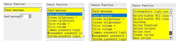
The sending message also assigns an ID of the sending message for sending a signal to the set ID. For example, the following figure is a list of alarm records. The sending message of the function key is set to ID=300, and all the clearing
