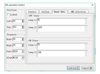
When select the characters displayed when the switch is in the state OFF/ON are determined by these two following attributes.
