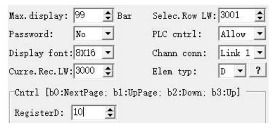
As shown in the figure: when D10=1, the alarm list page down; when D10=2, the alarm list is paged up;
