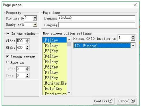
Whether modify the page to a window and the width and height, the back color and description can be decided here. (The current screen button setting function is not supported at this time)
