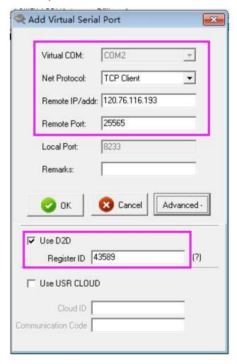
Note: network protocol select TCP Client; target IP/ domain name select 120.76.116.193 or coolmay.wicp.net (standby) (note: IP/ Domain name is coolmay domain name, need to link with coolmay server); target port select 25565; register ID in advance select 43589 (note: please set register ID after consult with coolmay technician)
