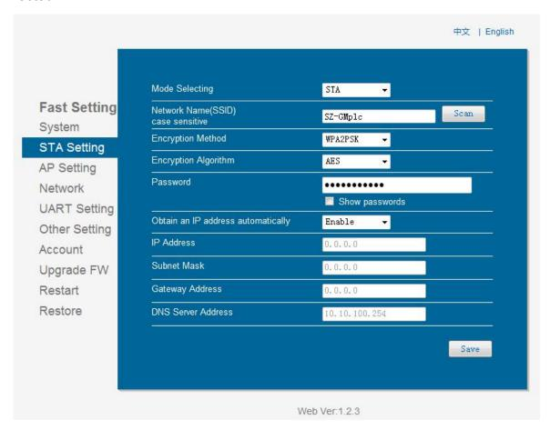
Select "SZ-GMplc" (Note: "SZ-GMplc" is the Internal wireless network of Coolmay), the setting of wifi hotspot will be introduced briefly. Click "confirm" after being searched and selected: the original name is changed.
