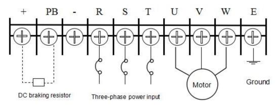
Figure 2-4 Main circuit terminal block wiring diagram
