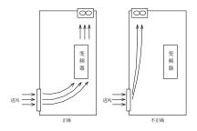
Figure 2-1 Fan position in the inverter installation environment
