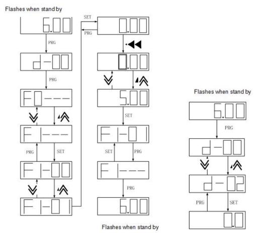
Figure 3-1 Flowchart for modifying function parameters
