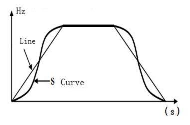
Figure 2 Acceleration and deceleration curves of the inverter
