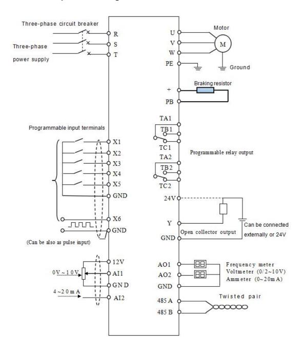
Figure 2-6 Basic operation wiring diagram
